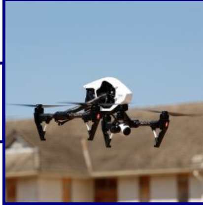
(left) The landing gear on this RPA raises to give the camera an unobstructed view
